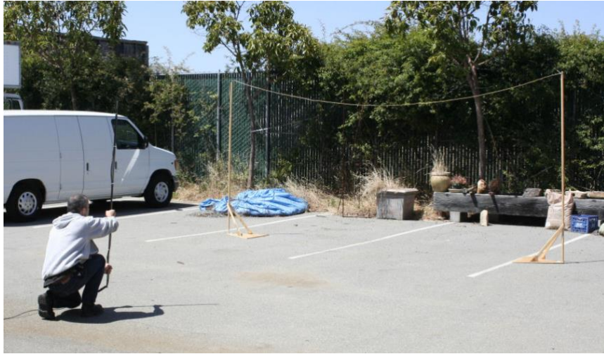
Figure 5. Test high voltage line. The wires were set at a 10 foot height.
